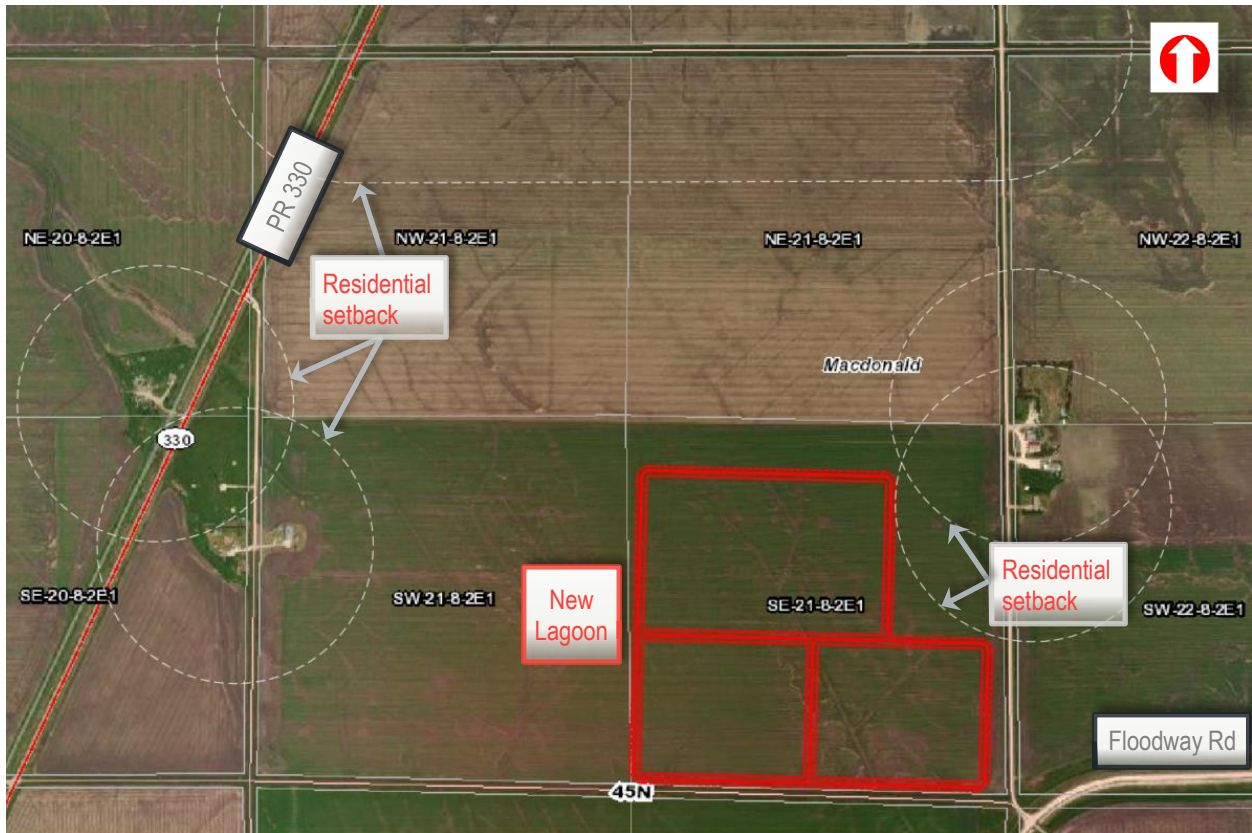
Figure 6-3: Option 3 New La Salle Lagoon Location and Sizing
