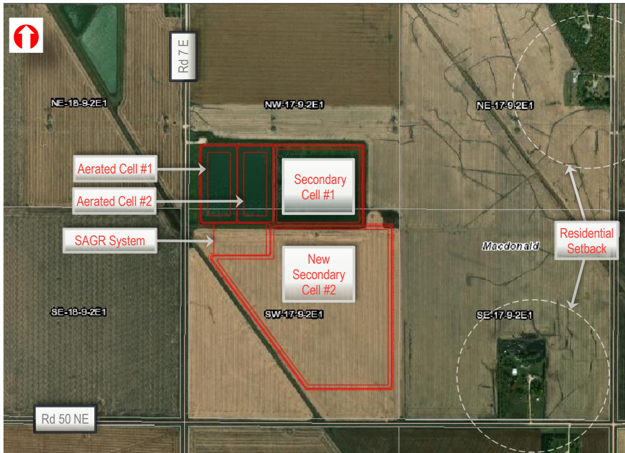
Figure 6-6 Option 5 – Oak Bluff Lagoon Expansion Configuration and Sizing
