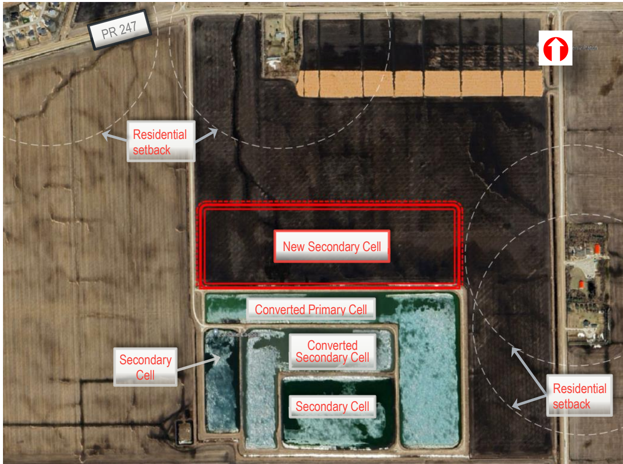
Figure 6-1: Option 1 Existing La Salle Lagoon Expansion
